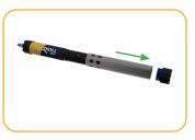
Remove restrictor from the instrument.
