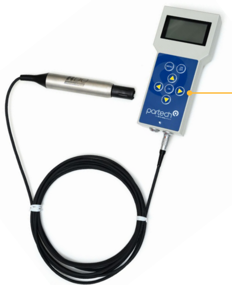
750 Portable Monitor with OxyTech RDO Sensor
