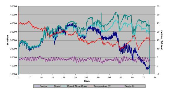
Figure 2: The control, one Aqua TROLL 200 Instrument with TROLL Shield guard, and one Aqua TROLL 200 Instrument with TROLL Shield guard and nose cone were tested side-by-side over an 81-day period.
