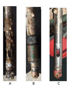
Figure 3: Three instruments after 81-day test. **Photo A**: Aqua TROLL® 200 control. **Photo B**: Aqua TROLL 200 with TROLL® Shield guard and nose cone still installed. **Photo C**: Aqua TROLL 200 with TROLL Shield nose cone in place and guard removed to show how effectively the guard protects the conductivity cell from biofouling. The conductivity cell was not cleaned.
