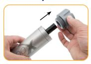
Remove nose cone from RDOX. Slide off RDO cap.
