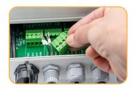
Thread wires through cable gland opening. Remove terminal plug from terminal block.
