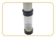
Put instrument in cup. Allow it to humidify for up to 5 minutes.
