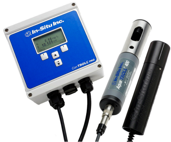
Figure 8. Both the Aqua TROLL 400 Multiparameter Instrument and the RDO PRO Probe connect to the Con TROLL PRO System for use in wastewater treatment plants and in recirculating aquaculture systems.
