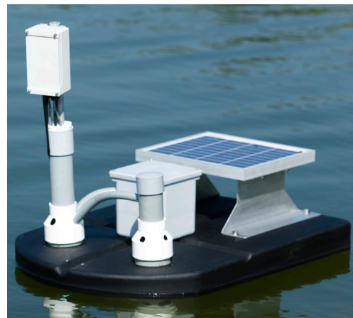
Figure 9. In-Situ wireless Aquaculture Buoy for inland fish production includes the RDO PRO Probe
