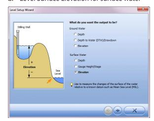
c. Level Surface Elevation for gage height/stage
