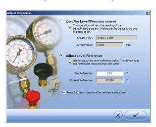
4. With the transducer in place in the water, enter the correct reference value and click the check mark.
