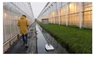
Figure 1. Mapping greenhouse discharge in the canal system
