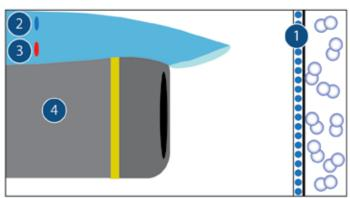
1. Oxygen-permeable sensing element contains lumiphore molecules
