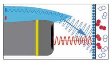
The optical RDO Sensor initiates a reading by sequentially turning on the blue and red LEDs. The blue light excites lumiphore molecules in the sensing element. The red light provides a zero phase reference. Excited lumiphore molecules emit red light. The photodiode detects both red returned light from excited lumiphore molecules and red reference light from the red LED. Optical electronics report dissolved oxygen (DO) concentration in mg/L.
