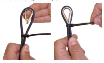
4. Place the second zip tie directly below the first and tighten.
