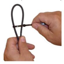
3. Place the metal loop inside the cable loop. Push the zip tie up to form a tight band around the metal loop. Tighten the zip tie.
