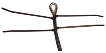
6. Hand-tighten the zip ties. Do not overtighten.
