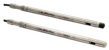
The Aqua TROLL 200 Instrument includes conductivity, level/pressure, and temperature sensors. The Aqua TROLL 100 Instrument includes conductivity and temperature sensors. Derived parameters available include actual conductivity, specific conductivity, salinity, total dissolved solids, resistivity, and density.
