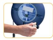
Use the cable reel handle to slowly lower the sensor into settling tank.
