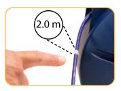
Record the sludge blanket's depth by noting the highest numerical measurement on the cable.
