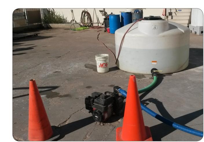
Figure 4. Injection Tank, Pump, and Piping
