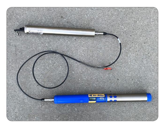
Figure 6. AquaTROLL 600 and TubeR Telemetry System
