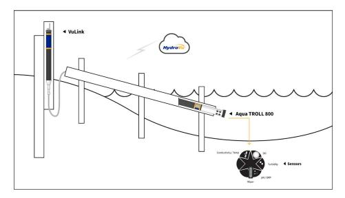
A sonde and tube deployment offers a cost-effective, low-maintenance installation option for CSO monitoring.
