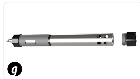
Flip restrictor and replace end cap before deployment.
