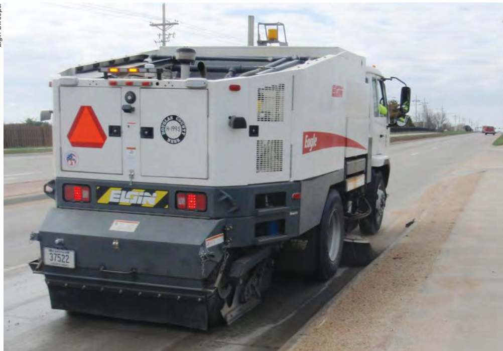
Each spring, road salt and sand are removed before road restriping begins.
