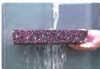
KBI Flexi-Pave™ Porous Pavement Allows Infiltration & Removes Pollutants
