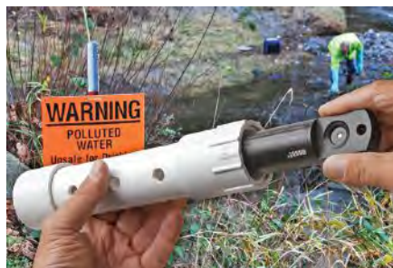
Protective housing for an underwater data logger
