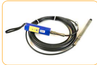
B. Instrument is ready to pair with software. Turn on the Wireless TROLL Com.
