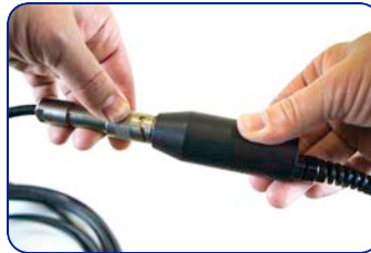
A. Connect Rugged Cable to TROLL Com and instrument.
