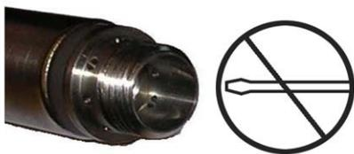
A TROLL pressure sensor with the nose cone removed. Do not insert **ANY** object into the sensor opening. Doing so voids the warranty.
