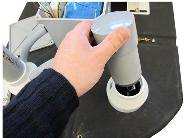
4. Put on gloves to handle the fiberglass drive shaft.
