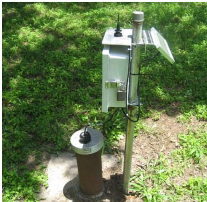
Figure 6: Level TROLL 500 Instruments log Lovelady monitor well every hour. A TROLL® Link Telemetry System transmits data to a cell phone at the main office.
