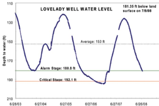
Figure 2: Level TROLL Instruments continuously collect data for the BSEACD. This hydrograph of Lovelady monitor well was developed using data collected with Level TROLL Instruments.
