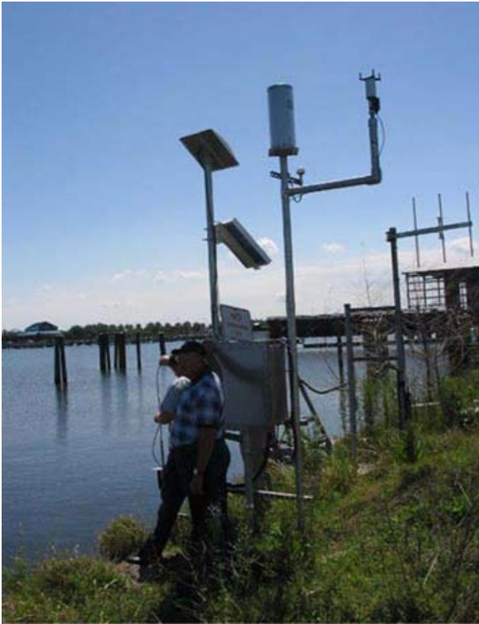
At Lakefront Airport monitoring station on Lake Pontchartrain, Bill Emmett inspects the system, which includes a Level TROLL® 500, solar-charged battery, GOES radio antenna, rain gauge, GPS antenna providing GOES timing documentation, and wind sensors. Emmett reported this location was under 10-15 feet (3-4.6 m) of water during Hurricane Katrina.
