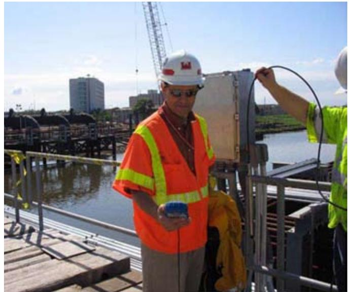
*George Brown of the USACE New Orleans District Water Management Office works with an In-Situ RuggedReader® Handheld PC and Aqua TROLL 200 Instrument at a pumping station on 17th Street Canal, constructed after Hurricane Katrina. The gates behind him were included in the new structure to control water surge into and out of the canal. The USACE has recently deployed Aqua TROLL 200 units to profile key water parameters along waterways in the New Orleans District.*
