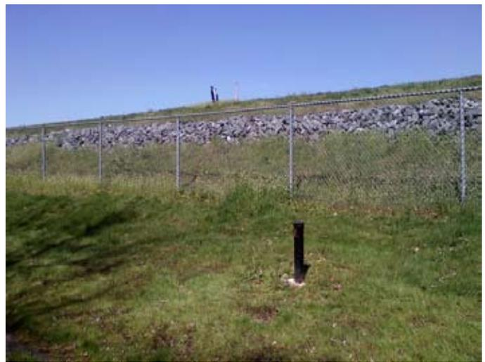
*Rugged TROLL® Instruments are deployed in off-site monitoring wells near a landfill to track groundwater levels.*
