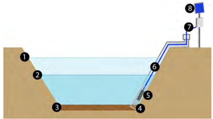
Natural pits, ponds, or other open-air impoundments are typically more complex due to their irregular shapes. These types of impoundments require calculation of the average depth and the surface area. Average depth is measured using a grid pattern covering the entire impoundment area. Record the depth measurements for each section of the impoundment. Add each measurement together and divide by the total number of measurements to calculate the average depth.
