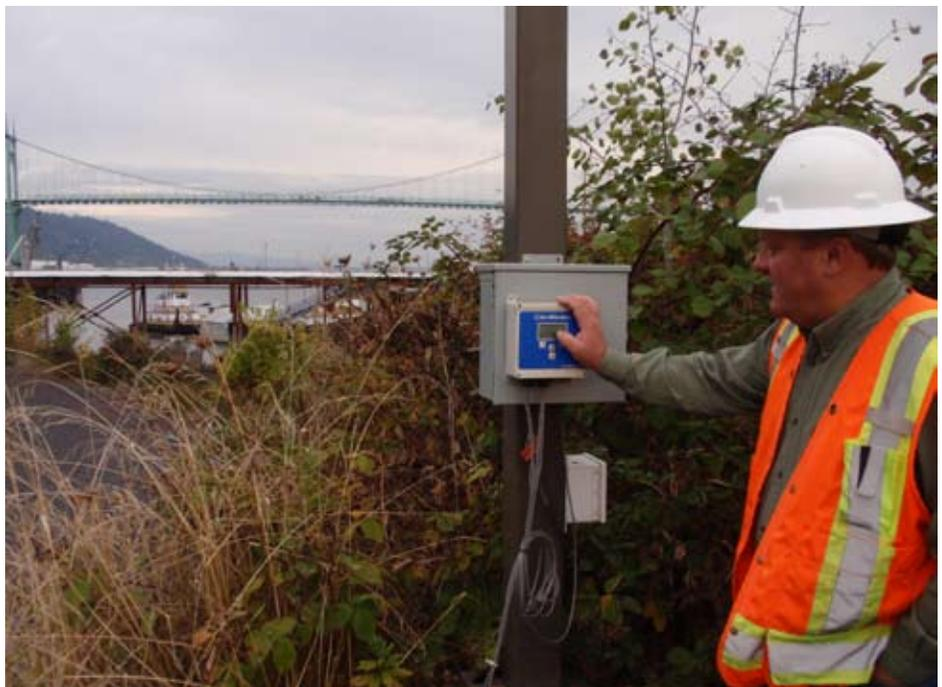
Stone checks water levels being reported by a Level TROLL 500 Instrument deployed in a monitoring well. The Con TROLL PRO System displays and records water level and temperature from up to two Level TROLL 500 Instruments, as well as ambient barometric pressure and air temperature. The Willamette River can be seen in the background.
