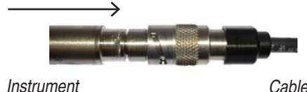
5. Slide the sleeve on the cable toward the instrument body until the pin on the body pops into the round hole in the slot on the cable connector.
