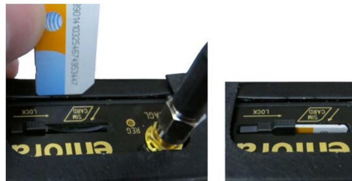
1. Align the SIM card so the diagonal cut is facing towards the antenna base.
