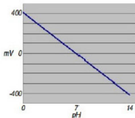
Figure 1. pH sensor calibration graph
