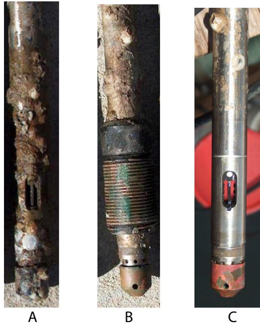
Figure 3: Three instruments after 81-day test. **Photo A:** Aqua TROLL® 200 control.
