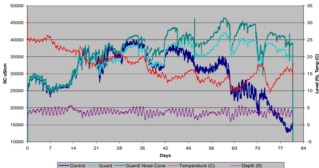
Figure 2: The control, one Aqua TROLL 200 Instrument with TROLL Shield guard, and one Aqua TROLL 200 Instrument with TROLL Shield guard and nose cone were tested side-by-side over an 81-day period.
