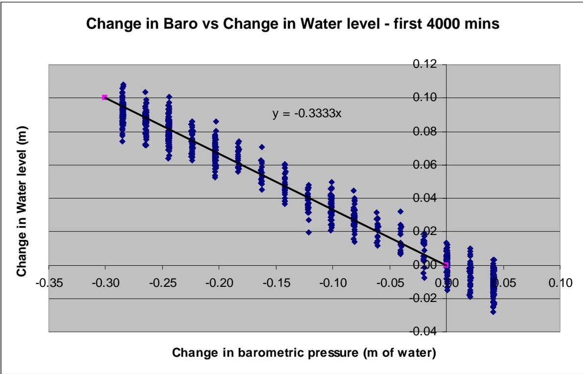
**Figure 3 Water level - barometric correlation showing 33% BE**
