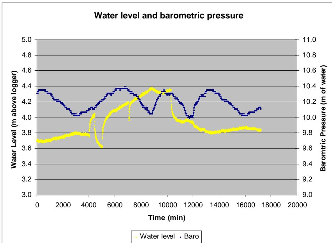
Figure 2 Water level above logger and barometric data record
