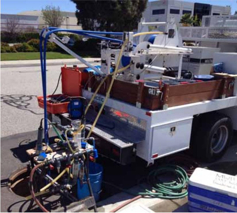
Figure 2. The WRD staff simultaneously run two smarTROLL Low-Flow Systems to save time at sampling events.
