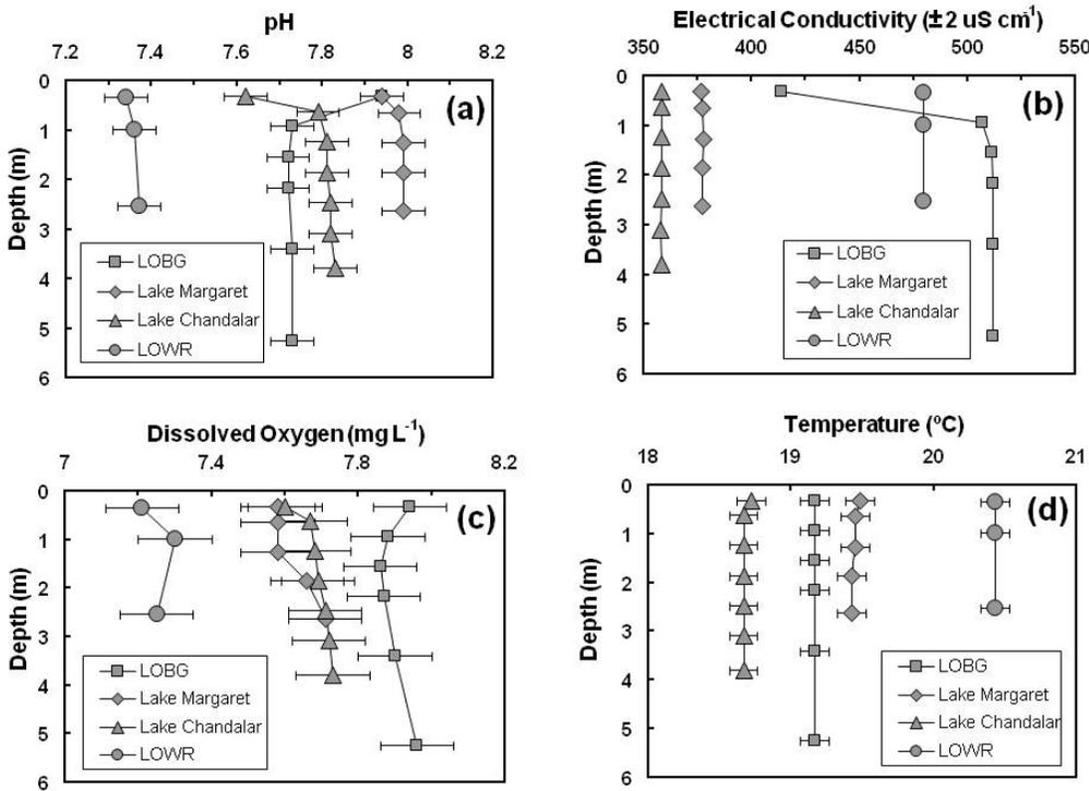
Figure 1. Chemical profiles for pools studied: (a) pH, (b) electrical conductivity, (c) dissolved oxygen, and (d) temperature. Error bars represent the accuracy of measurement for each TROLL 9500 sensor.
