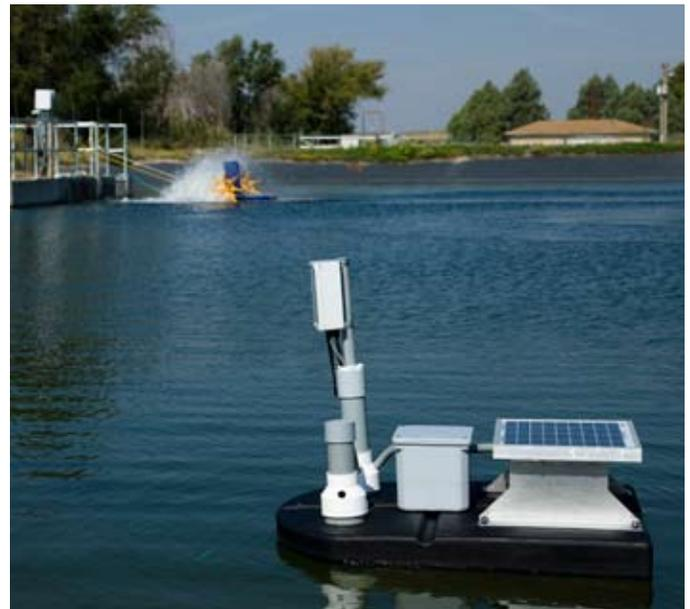
*Wireless monitoring buoy measures oxygen. Relays power on aerators as needed.*
