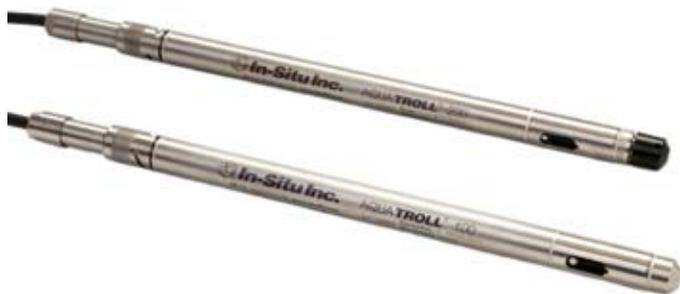
The Aqua TROLL 200 Instrument includes conductivity, level/pressure, and temperature sensors. The Aqua TROLL 100 Instrument includes conductivity and temperature sensors. Derived parameters available include actual conductivity, specific conductivity, salinity, total dissolved solids, resistivity, and density.
