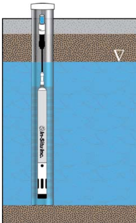
Figure 1. Vented sub-2" TROLL 9500 with pH, temperature, conductivity, and RDO sensor. Attach RuggedReader handheld PC or laptop via TROLL Com when downloading data.
