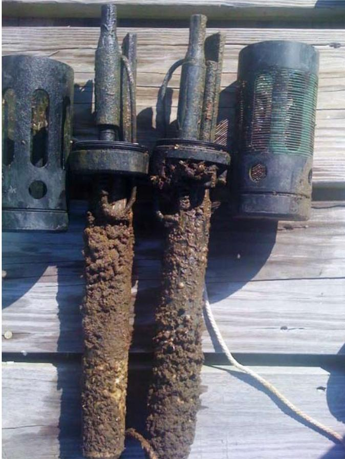
Figure 11: Control instrument (left) and experimental instrument (right) deployed at Site #3
