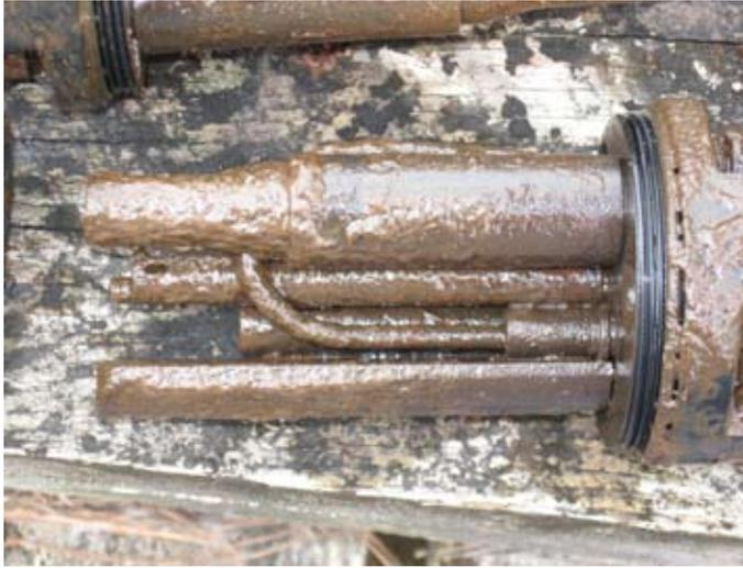
Figure 14: Control instrument after two-month deployment at Site #4
