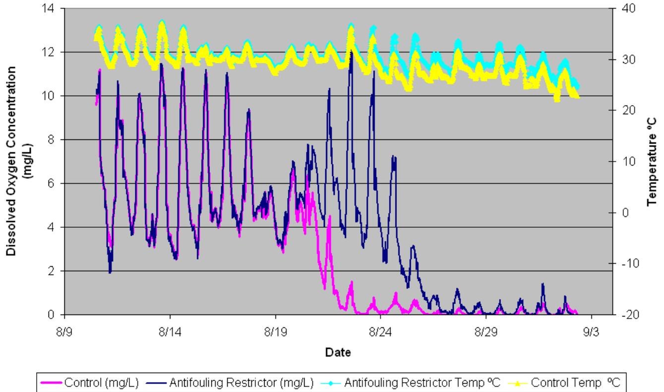
Figure 6: This graph compares DO readings for both control and experimental instruments deployed at Site #2. The experimental instrument with the TROLL Shield Guard increased deployment time by one week over the control unit.
