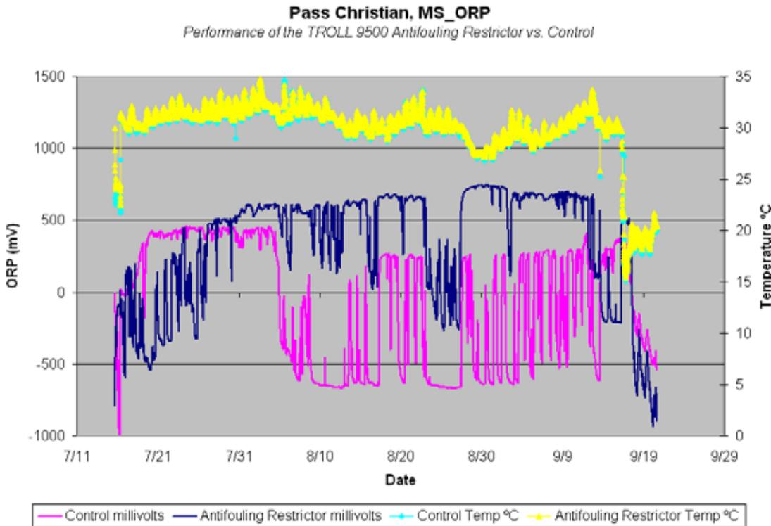
Figure 10: The graph compares ORP readings collected by both control and experimental instruments at Site #3. Fouling on control sensors resulted in an offset for the duration of deployment.
