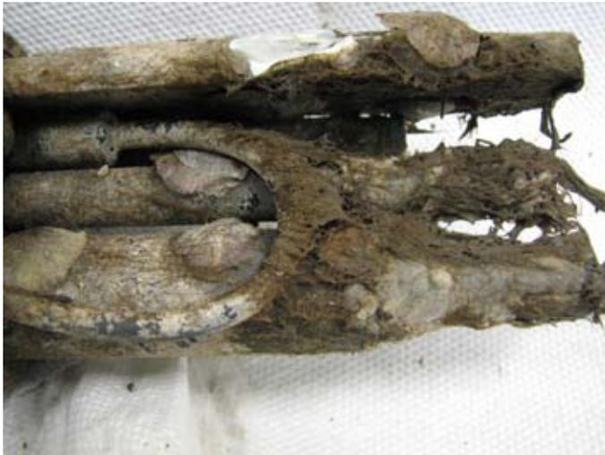
Figure 7: Sensor fouling on the control instrument after 25 days at Site #2
