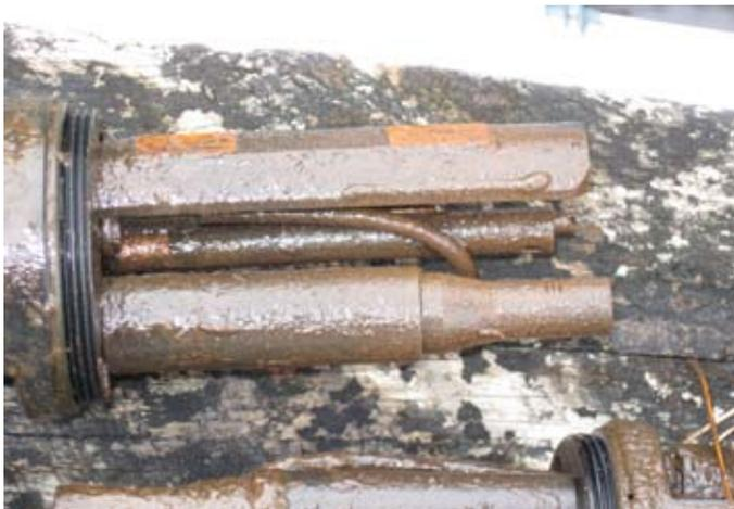
Figure 15: Experimental instrument after two-month deployment at Site #4
