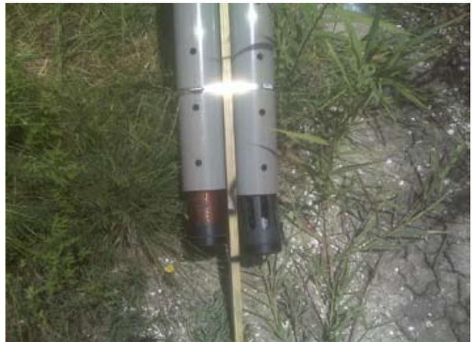
Figure 5: Control instrument (right) and experimental instrument with TROLL Shield Guard (left) being deployed at Site #2.
