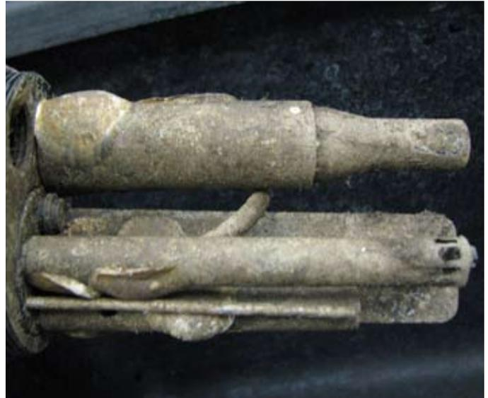
Figure 8: Sensor fouling on the experimental instrument after 25 days at Site #2
