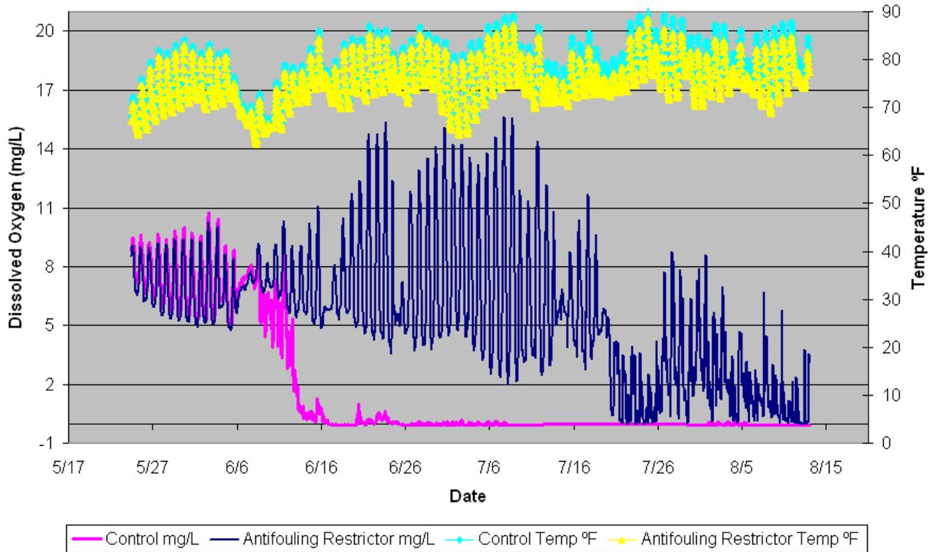
Figure 3: This graph compares DO readings for both control and experimental instruments deployed at Site #1. The experimental instrument with the TROLL® Shield Guard collected data for six weeks longer than the control unit.
