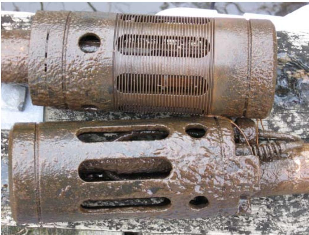
Figure 13: Control instrument (bottom) and experimental instrument with TROLL Shield Guard (top) deployed at Site #4
