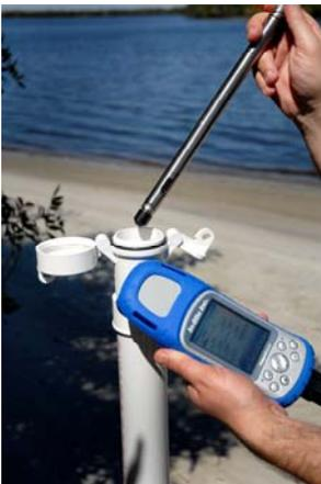
The In-Situ Aqua TROLL® 200 instrument (see Figure 1) monitors and records water level, temperature, plus conductivity and salinity. The Aqua TROLL 200 instrument automatically and continuously corrects its depth and level parameters for changes in water density due to changes in salinity. This can dramatically improve the accuracy of depth and level measurements in estuaries and coastal waters where tides and rainfall continuously affect the local salinity.
