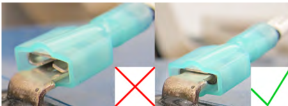
Figure 2.11 Incorrect and correct battery connection
