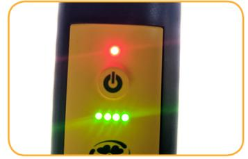
The device lights will turn on and blink according to charge level.
