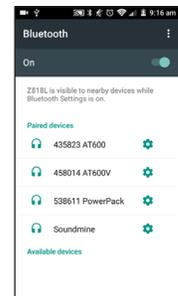
From device's Bluetooth Settings screen, tap serial number of Wireless TROLL COM and then tap the device's back button.
