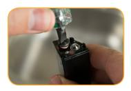
Remove sensor from sonde and unscrew reference junction.
