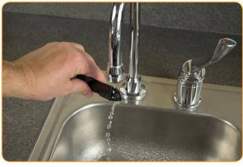
Soak overnight for the best long-tem results. Rinse thoroughly with deionized water prior to calibration.
