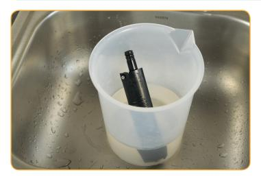
Soak sensor for a minimum of two hours in 355 mg/L chloride standard or the highest standard you plan to use during calibration.
