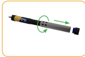
Remove restrictor from the instrument.
