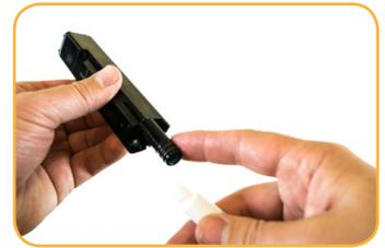
Lubricate o-ring at bottom of sensor.
