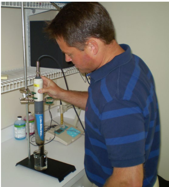
Figure 4. Mike Piehler calibrates the TROLL® 9500 Water Quality Instrument in the laboratory before deploying it to an outfall monitoring site.
