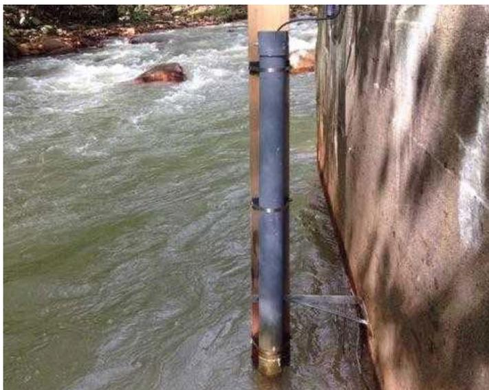
**Figure 5.** Aqua TROLL 600 deployed in a stilling well at the mouth of Muddy Creek.
